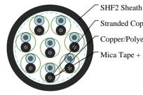
SHF2 Sheath Stranded Copper Conductor Copper/Polyester Tape + Drain Wire Mica Tape + HFEPR Insulation
